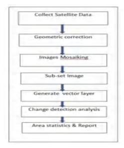
Figure 21: Flow chart of methodology used for processing images.
